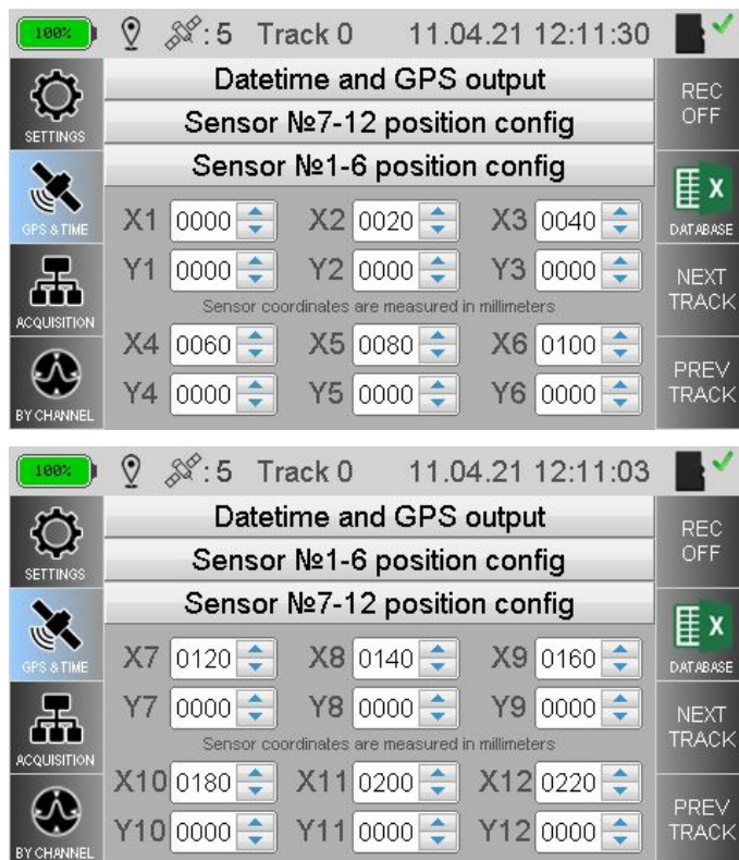
Fig.4.11. Magnetic measurement unit positions of the multichannel metal stress scanner configuration page
