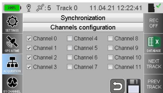
Fig.3.13. Panel for enabling and disabling recording of measured signals of multichannel scanner to file by channel
