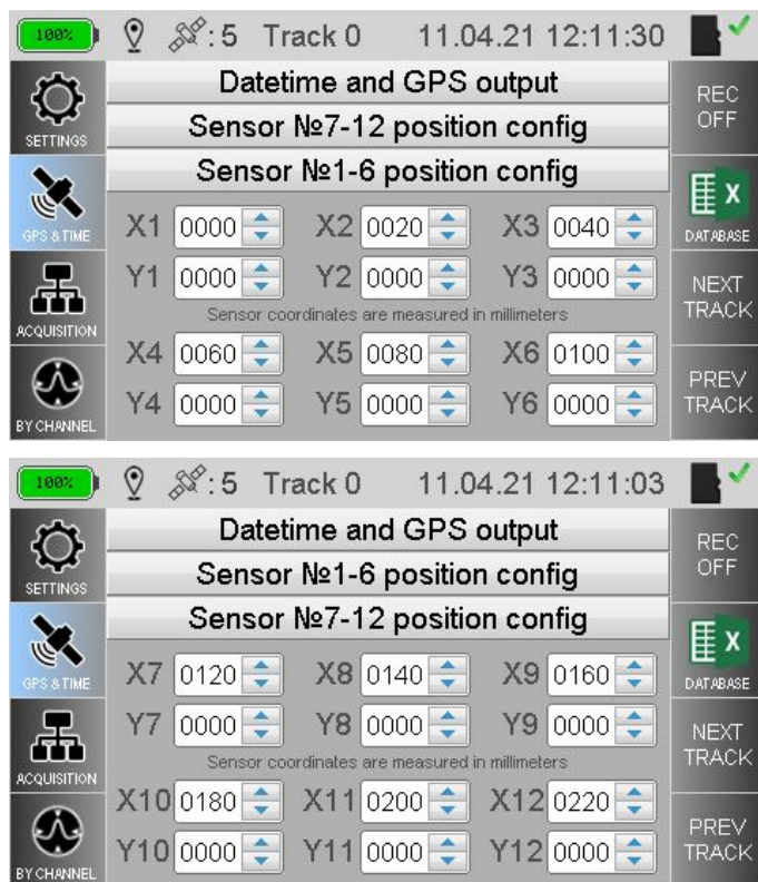
Fig.3.11. Explaining the magnetic measurement (scanning) unit positions configuration page
