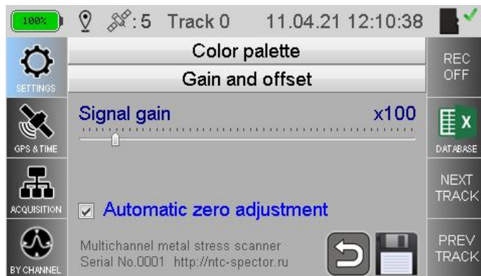
Fig.3.9. Amplification factors and zero offset adjustment panel for gradiometer (top) and 3-axial topology (bottom) magnetic field sensor units
