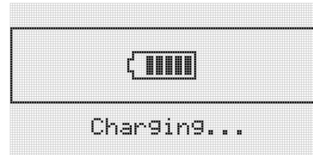
Fig.3.8. Indication of the battery charge process on the IN-02 stress scanner screen
