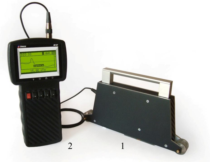
Fig.3.2. Appearance of IN-02 the metal stress scanner 1 – magnetic measuring unit, 2 – electronic unit.
